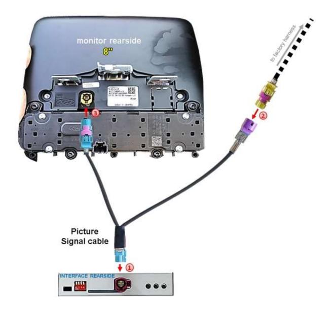
After installing the interface in between and power is on, the OEM image should be shown on screen.
