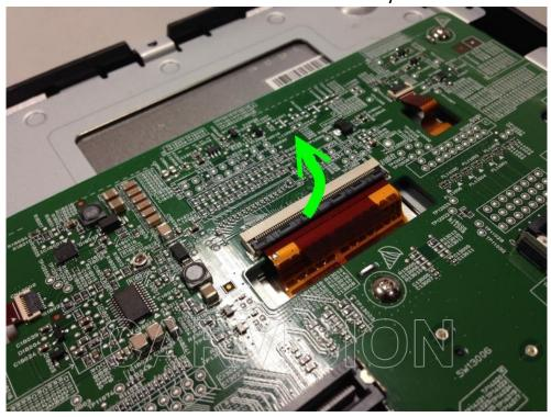
Remove the "ears" of the original cable to make it straight
