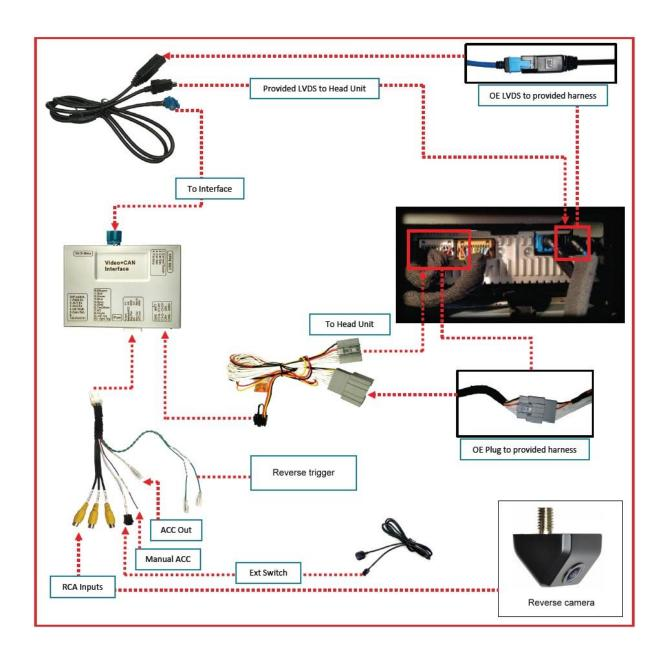
Optional ACC OUT wire: 12V power signal (for example to power the rear cam).
