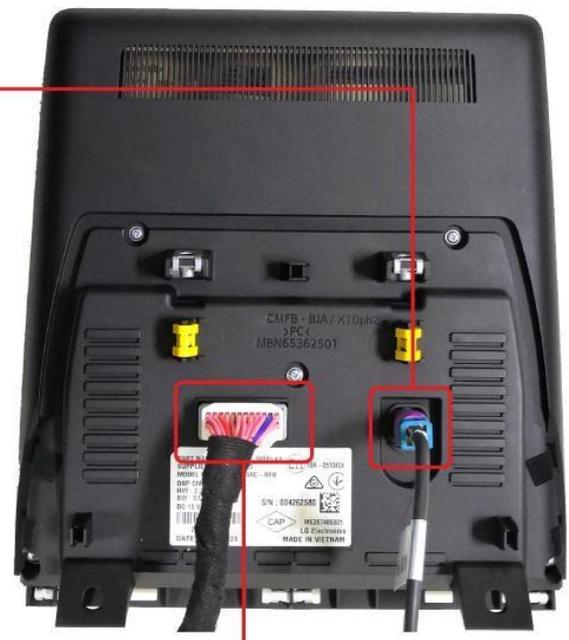
This Power harness should be installed behind the screen
