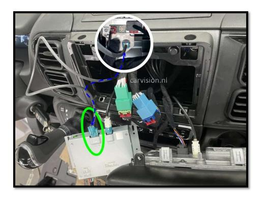
Power/CAN: connect the plug&play power harness (blue + green) between the head-unit and car wiring harness.
