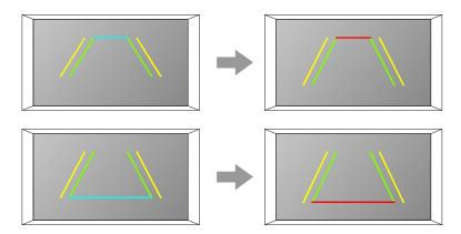
• Press "center" to select the up/down line, the color of blue line turns red, then adjust it by pressing "left" or "right", after that press "center" to save the parameter.
