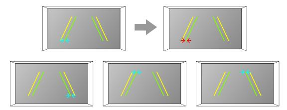
• Complete the angle of vehicle line marks setting, then press "right" to enter detection zone adjustment interface, press "center" to select the arrow, the color of arrow turns red, then adjust it by pressing "left" or "right", after that press "center" to save the parameter. Repeat the same procedures to adjust the other arrows.
