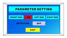
Press "right" button to move the cursor to the LDW, then press "center" to enter the parameter adjustment interface.
