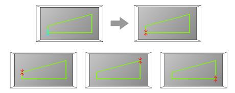
• Press "left" or "right" to select up/down/left/right lines, press "center" to enter the adjustment interface, the color of blue line turns red, then adjust the position of the line by pressing "left" or "right", after that press "center" to save the parameter. Repeat the same procedures to adjust the other lines.
